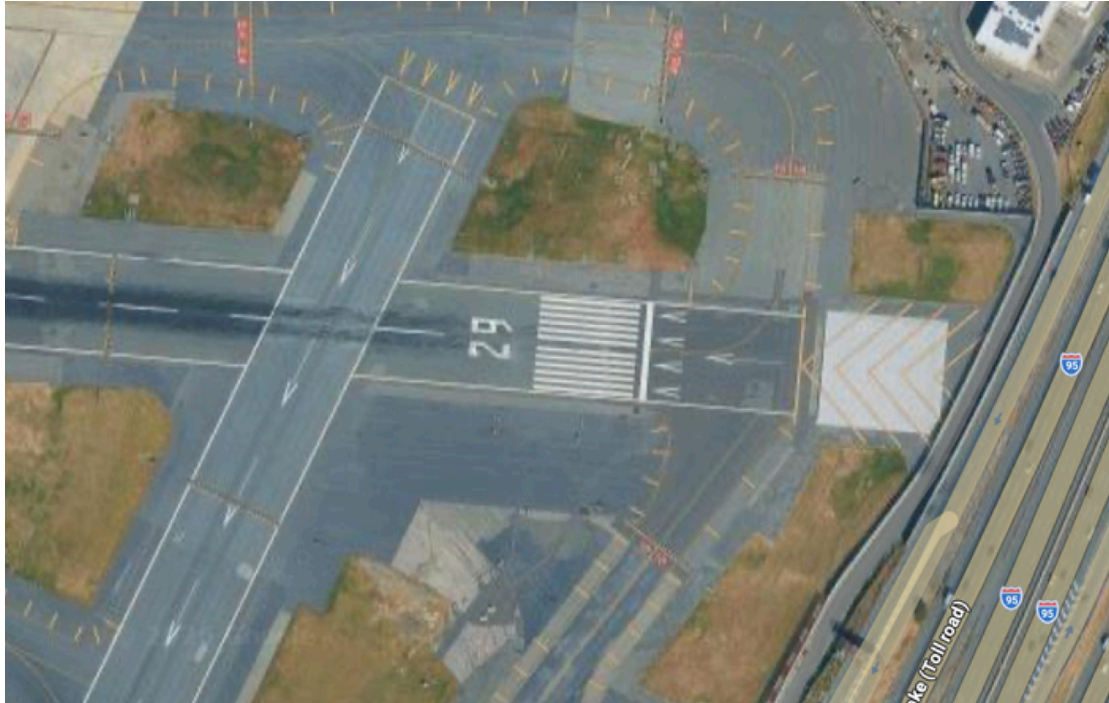
Runway at Newark. EMAS and displaced thresholds RWY 29 and RWY 22R.
